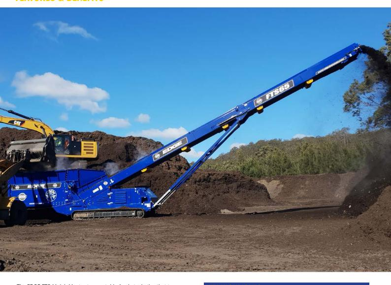
The EDGE FTS Mulch Master is a portable feed stockpiler that is specifically designed for the stockpiling of lower density, bulky materials such as mulch, compost and soils. The EDGE FTS Mulch Master combines traditional flipping and rotation with constant material flow to provide blockage free stockpiling whilst also preventing compaction, contamination and risk of combustion. It can accept material directly fed from wheel loaders, wood grinders, shredders, screeners or trommel screens.
